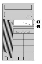
Figure 24. Removing the card reader cover
